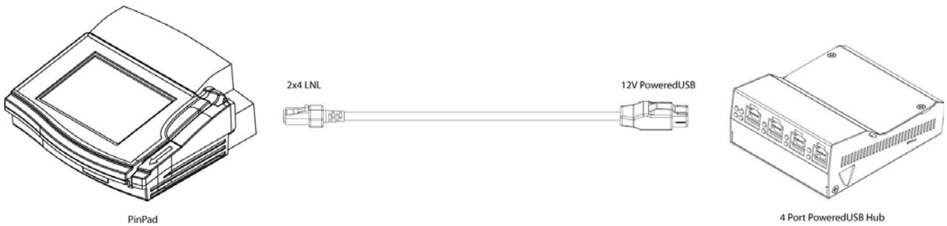
Figure 2-9. Cables; +12V PoweredUSB to +12V Power Jack and RS-232 to RS-232
